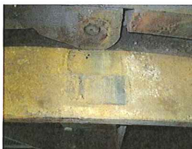
Example of Wear to Radius Arm from Bushes
