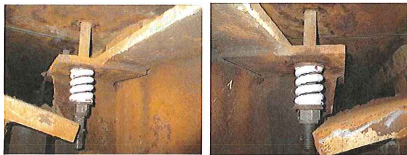
New springs fitted to tongue plate
